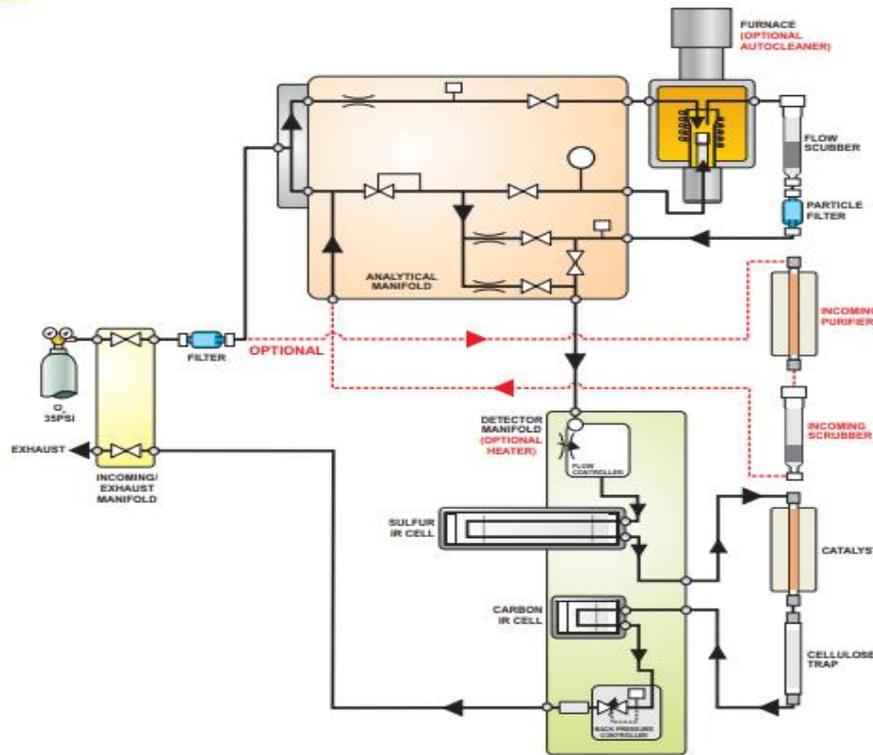
Figure 4:Flow diagram showing Carbon/Sulfur Analysis process from LECO Corporation
