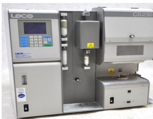
**Figure3:LECO CS230 Analyzer for Total Organic Carbon**
